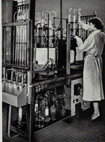
A routine measurement on a wave guide component of a linear accelerator used in the X-ray treatment of cancer.
