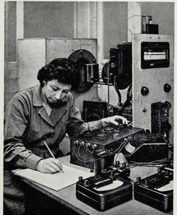
Measurement of the thermal conductivity of a semi-conducting material
