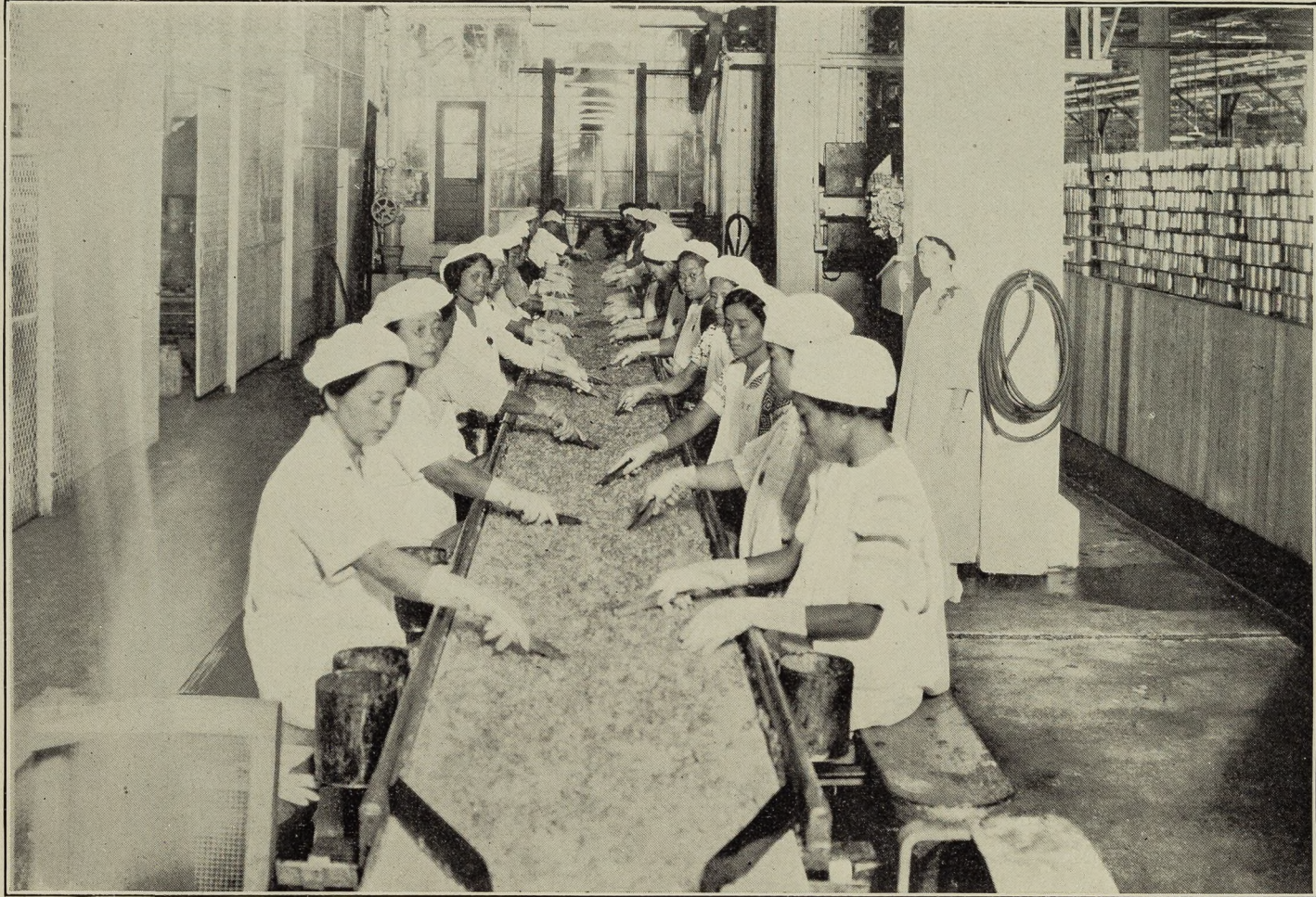
PLATE 6.—REMOVING BITS OF SHELL FROM CRUSHED FRUIT
