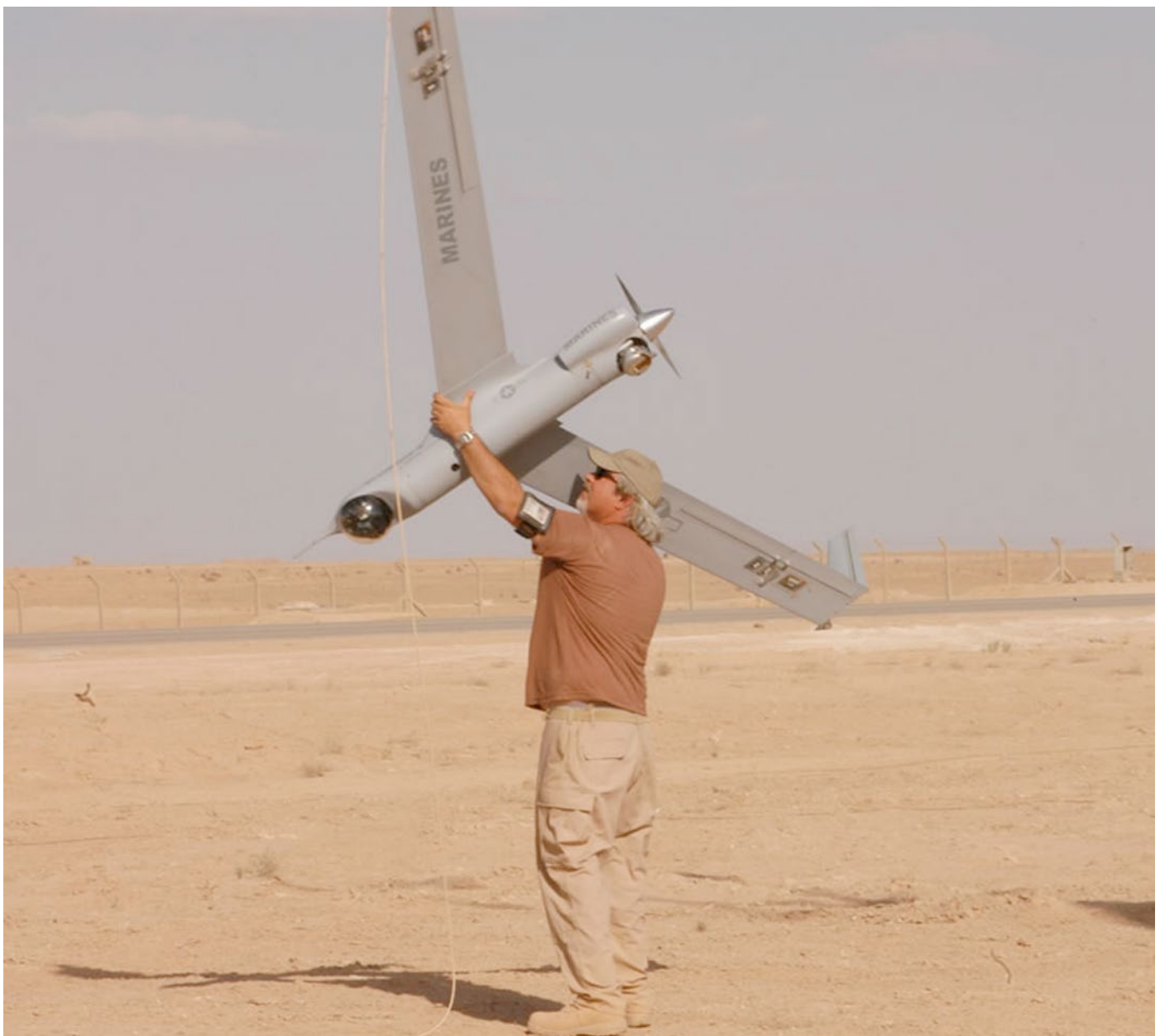
The ScanEagle, launched by a catapult, flies either preprogrammed or operator-initiated missions. Source: http://media.defenceindustrydaily.com/images/AIR_UAV_ScanEagle_Recovered_Ig.jpg
