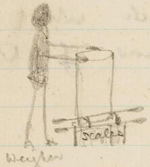
truck, steps & van on one level. The weigher then stands on the platform of the steps, & the process of filling goes on as before.
