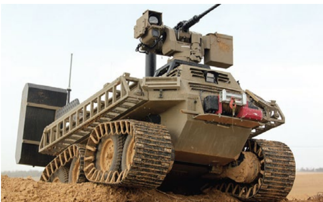
Image of Guardium semi-autonomous unmanned ground system taken from G-NIUS product brochure
