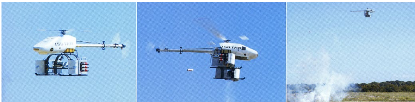
Aero Cougar system being carried and fired from a UAV, images taken from Ettiene Lacroix Group/Alsetex Aero Cougar brochure, distributed at MILIPOL 2015
