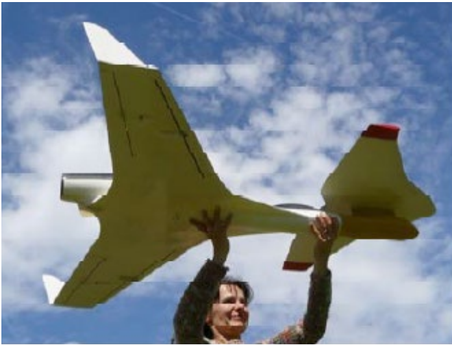
Airborne Long-Range NLW Dispenser, image taken from NATO RTO report, April 2012, original source Fraunhofer-Institut für Chemische Technologie
