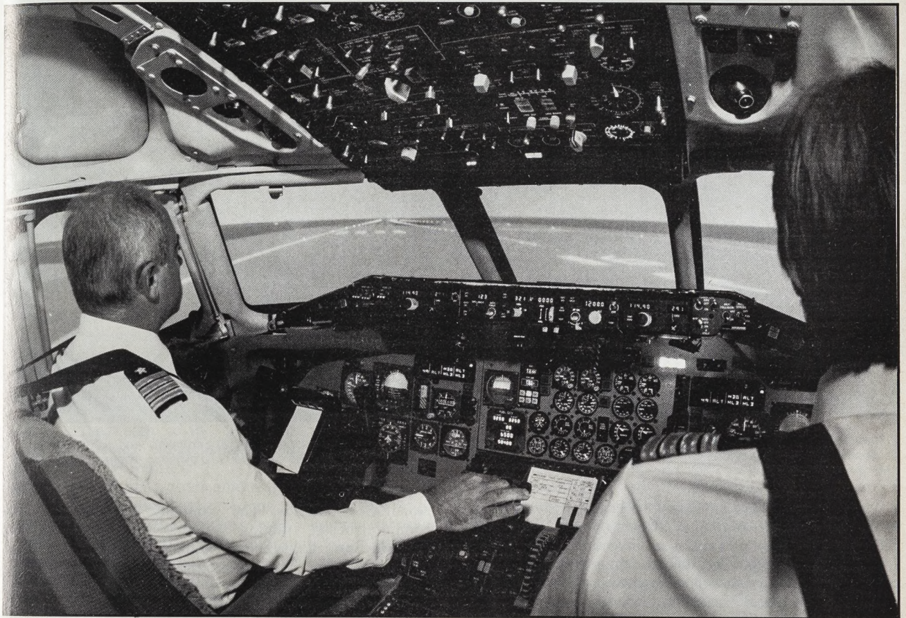
Alitalia MD Super 80 flightdeck with 'wide' display and Novoview SP3 visual simulation.
