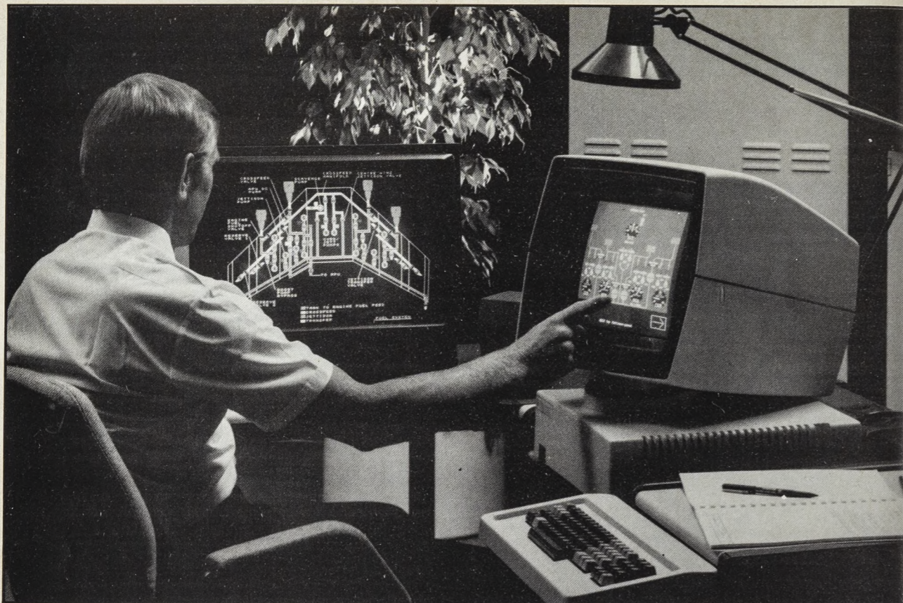
Photo: Rediffusion Simulation Ltd Interactive training systems translate conventional training programmes into dynamic self-teach lessons stored in a computer and accessed through a keyboard and touch sensitive screen. Here a simulated Boeing 747 flight deck panel is linked through the computer, to a dynamic schematic of the aircraft's fuel system.
