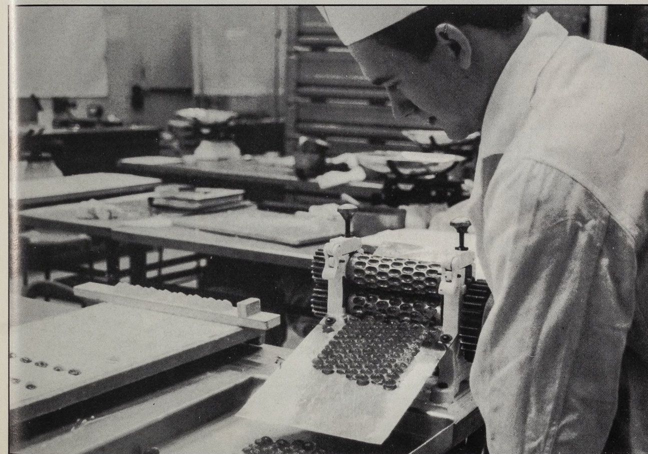
Boiled sweets being moulded by Robert Crowe, APV Baker plc, using a drop roller at the Polytechnic of the South Bank.
