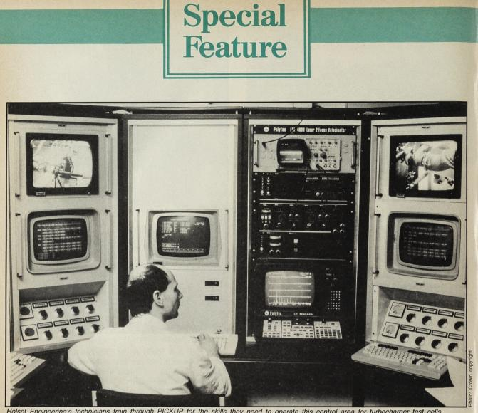
Holset Engineering's technicians train through PICKUP for the skills they need to operate this control area for turbocharger test cells
