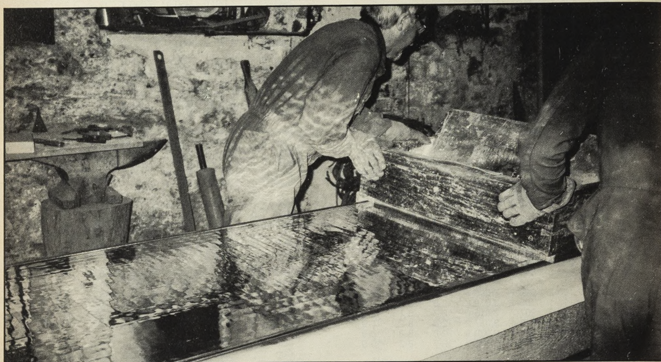
Production of lead sheets. At this stage the sheet is still fluid.
