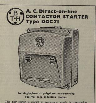
This new starter is elegant in appearance, sturdy in construction, and dependable in operation. It is available for motors up to 5 horse-power, and complies with BS.587 for "Frequent Duty", i.e. forty starts per hour. The starter, comprising a triple-pole contactor with normally-open auxiliary switch and triple-pole hand-reset thermal overload relay, is enclosed in a distinctive die-cast aluminium case with integral START-STOP push buttons.
