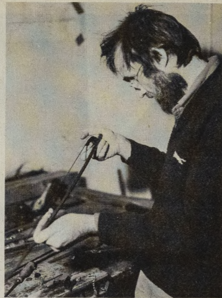
Mr Ken Cameron at work on a violin bow. One bow can take up to three days to make and only top quality woods and real horsehair are used.
