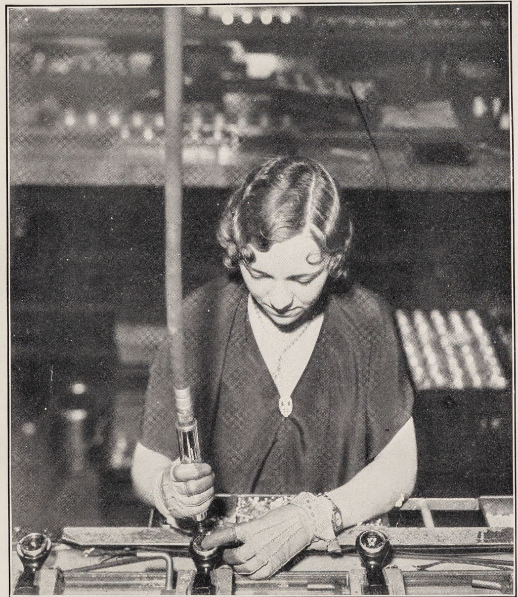
FLEXIBLE-SHAFT POWER SCREWDRIVER ON ASSEMBLY CONVEYOR.
