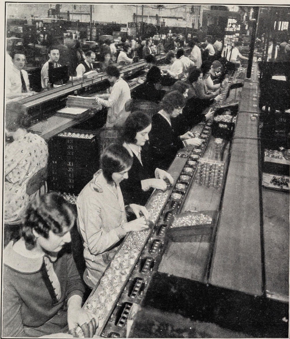
ASSEMBLING TELEPHONE RECEIVERS ON ASSEMBLY CONVEYOR.
